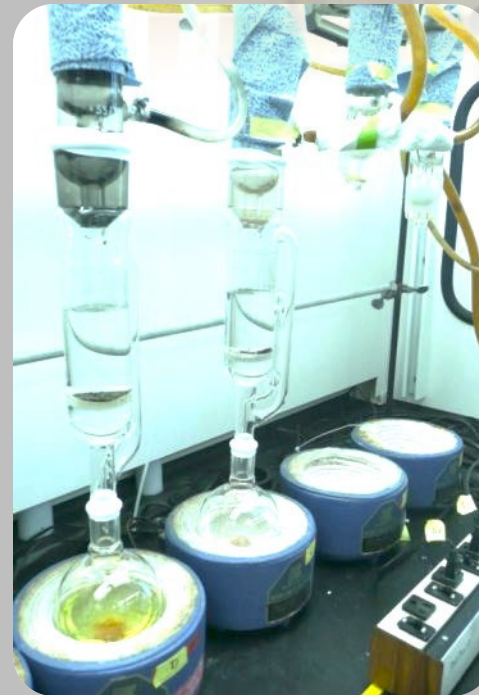
Soxhlet extraction setup for elemental S
